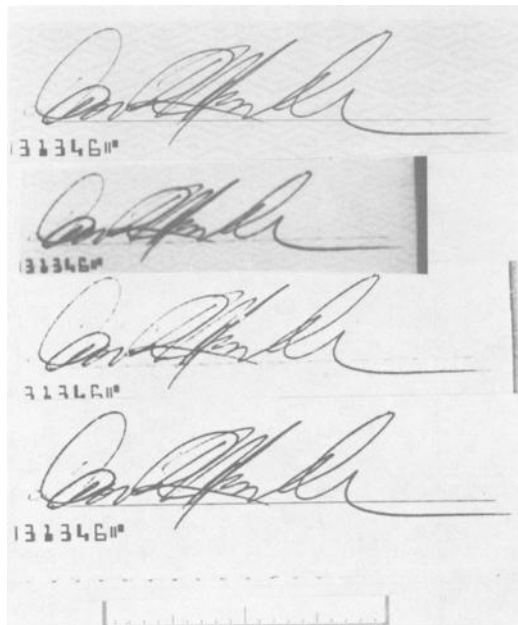
FIG. 2—Ballpoint pen (black ink). The first sample is the original "Duane R. Mueller" signature, the second sample is a thermographic copy (reduced \times 50 then retrieved at \times 43 ), the third sample is an electrostatic copy, and the fourth sample is a photocopy (electrostatic process).
