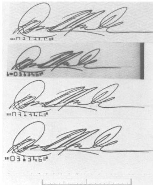
FIG. 4—Roller pen (black ink). The first sample is the original "Duane R. Mueller" signature, the second sample is a thermographic copy (reduced \times 50 then retrieved at \times 43 ), the third sample is an electrostatic copy, and the fourth sample is a photocopy (telectrostatic process).
